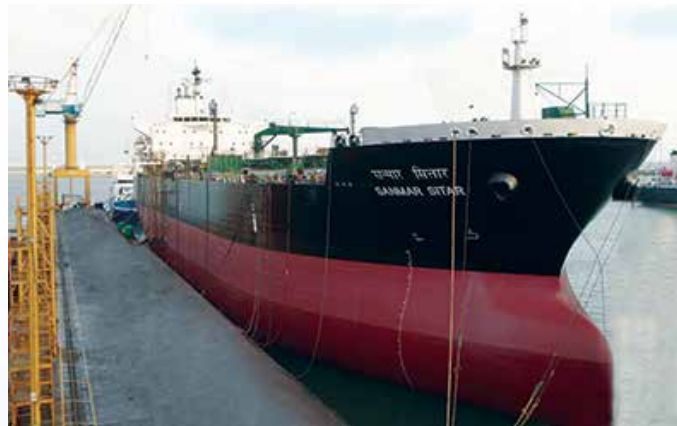
Sanmar Sitar - Double Hulled Oil Tanker, 48,700 DWT
