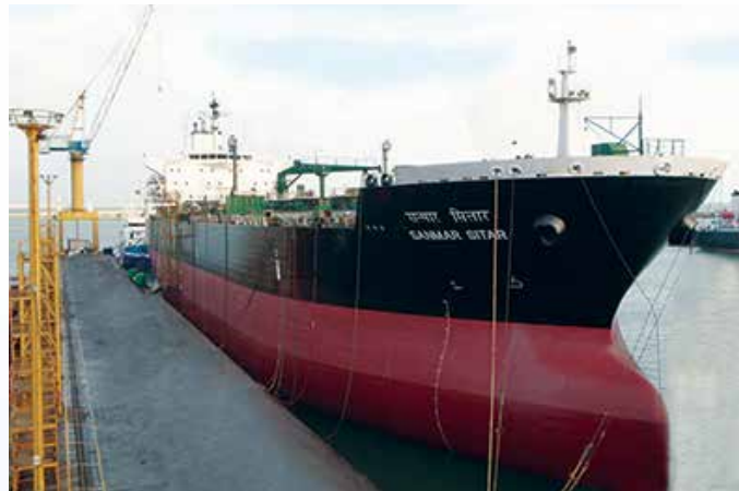
Sanmar Sitar - Double Hulled Oil Tanker, 48,700 DWT
